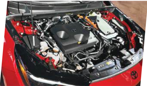
2.5-liter four-cylinder engine combined with Toyota's fifth-generation hybrid system (HEV)
